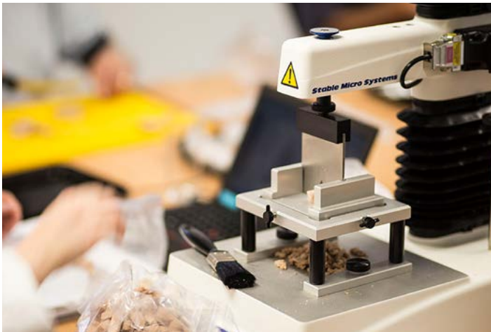
Shear force testing to assess tenderness of cooked meat samples
